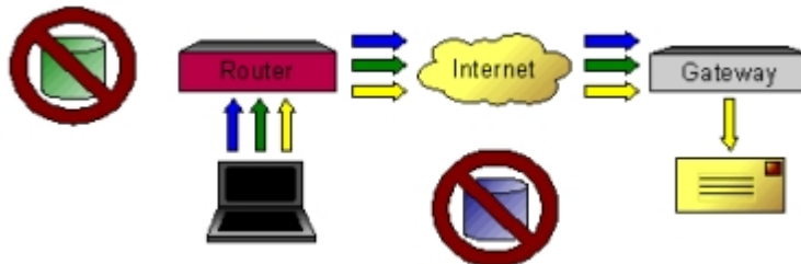
An example of a VPN Client that attempts to tunnel all traffic to the VPN Gateway.
